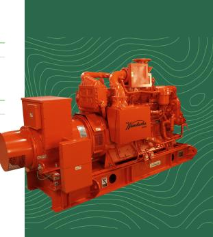
The Waukesha<sup>®</sup> VGF<sup>®</sup> generator sets offer a compact, fuel-flexible package delivering exceptional performance in prime power, cogeneration, peak shaving and stand-by power applications. The VGF24 generator set is designed for standby and continuous power applications and is rated at 325-360 kWe at 50 Hz (1500 rpm) and 390-425 kWe at 60 Hz (1800 rpm).
