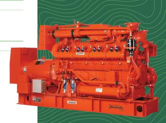
The Waukesha® VGF® generator sets offer a compact, fuel-flexible package delivering exceptional performance in prime power, cogeneration, peak shaving and stand-by power applications. The VGF48GSID generator set is designed for standby and continuous power applications and is rated at 610-685 kWe at 50 Hz (1500 rpm) and 730-825 kWe at 60 Hz (1800 rpm).
